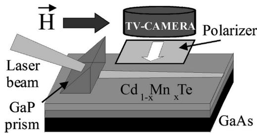
FIG. 1. Experimental setup to evaluate magneto-optical TE–TM waveguide mode conversion and optical propagation loss.
